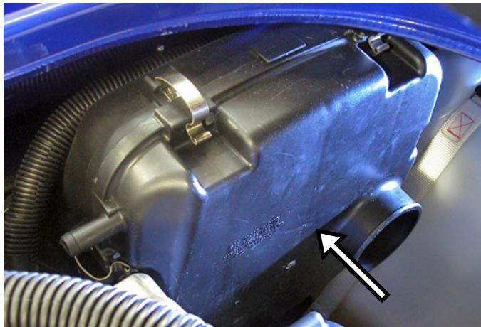
Remove air filter case mounting bolts (4 total – 2 on each side) and then air filter case. Discard bolts and case.
