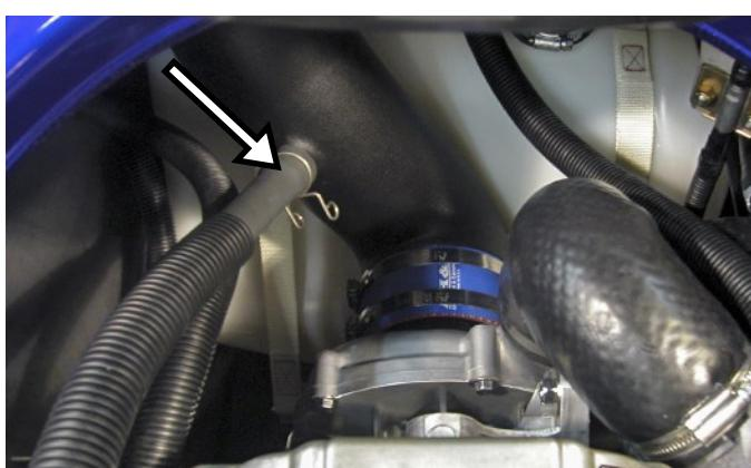
Secure using stock spring clamp.
