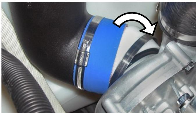
Install by rotating Power Filter tube assembly while pulling towards engine. NOTE: Tapered plastic flange installs into Power Filter tube.
